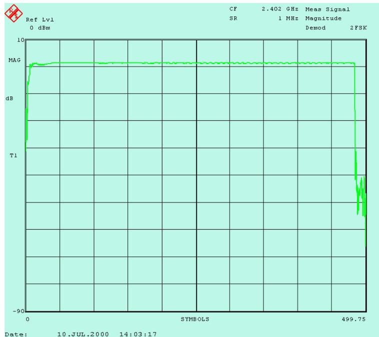
Bild 16 Modulation Characteristics: Magnitude
